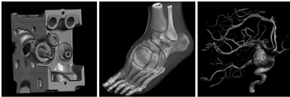
FIGURE 46.35 Various applications of lens-based distortions: ( left ) Magnifying inside features in an arbitrary-shaped area on an engine, ( middle ) applying a sampling-rate-based lens on a foot dataset, ( right ) enlarging an area of interest of an aneurysm. (See also color insert).
