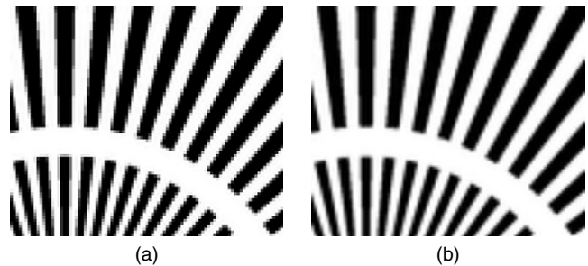
FIGURE 46.3 Magnification via interpolation with (a) a box filter; and (b) a bi-linear filter. The latter gives a much more pleasing result.
